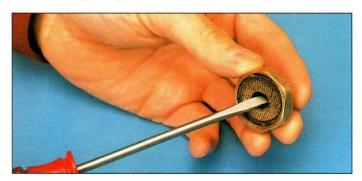
**Packing washer.** With the packing nut removed from the stem, the packing washer will be exposed. If the washer is jammed into the nut, pry it out with a screwdriver.
